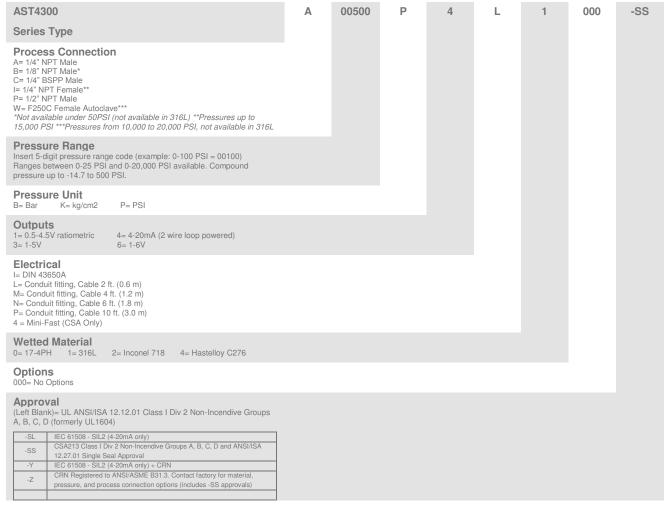
Note: CSA approved products require case/earth ground electrical connection. See wiring installation sheet for further details
