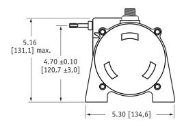
\* tolerance = +.005 -.001 [+.13 -.03] \*\* tolerance = +.005 -.005 [+.13 -.13]
