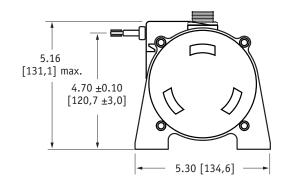
DIMENSIONS ARE IN INCHES [MM] tolerances are 0.03 IN. [0.5 MM] unless otherwise noted.
