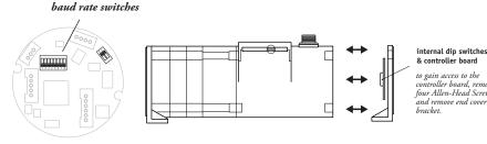
controller board, remove four Allen-Head Screws
