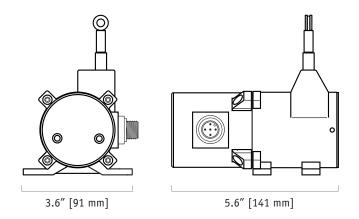
The PT8DN, using a high cycle plastic-hybrid potentiometer, communicates via DeviceNET protocol with programmable controllers in factories and harsh environments requiring linear position measurements in ranges up to 60".
