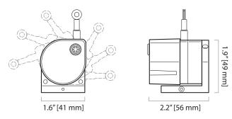
The MT2E is our new encoder-based member to our family of rugged, accurate miniature cable-extension position transducers. The Celesco MT2E features a highly-tensioned heavy-duty measuring cable that was designed for the high-acceleration demands encountered in flight testing and automotive crash tests.
