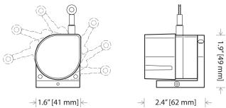
The MT3A is the solution for high-acceleration test applications in potentially wet environments. Just like the MT2A, the MT3A comes in 4 different full-stroke ranges, has a high-tension heavy-duty measuring cable designed for the demands of flight and automotive crash tests and comes with an easy to use 2-axis 360° rotation mounting bracket for installation in hard to fit areas.
