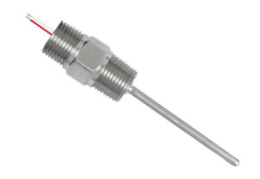
The Direct Immersion RTD Probe-win Threaded Fitting is constructed with a stainless steel sheath and a welded connection. The welded connection is typically a 1/2" x 1/2" NPT. 1/2" x 3/4" NPT or 3/4" x 3/4"NPT connection. The connection is dual threaded for use with a connection head. The sensors are available with single or dual junctions. These sensors are ideal for the process industry where immersion in the application is essential.
