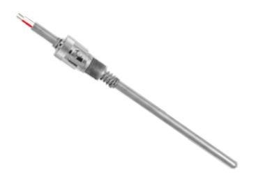
The **Spring Loaded Thermocouple Probe–Bayonet** is constructed with a stainless steel sheath and a bayonet fitting. Bayonet mounting provides a simple and inexpensive spring loaded option for installing probes where a fluid seal is not required. We also offer a 1/8" NPT mounting adaptor to assist with locking the sensor in position.
