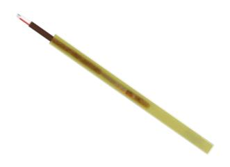
The **Stator Thermocouple** is a rectangular, flat, laminated sensors commonly called "Stator Sticks" because they are inserted between the coils in the stator of a motor. These sensors are used in electric motors and generators for continuous sensing of the temperature and provide for consistent thermal monitoring without false alarms. Measurement Specialties' Stator Thermocouples are built to meet the specifications of ANSI C50.10-1990, general requirements for synchronous motors.
