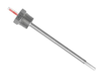
The Point Sensing RTD Probe—Process Threaded Fitting is constructed with a rigid stainless steel sheath with an element embedded into an aluminum tip. The aluminum tip provides faster time response. These sensors are typically designed for use in plenums and ducts within HVAC systems. They can also be utilized whenever a quick time response in a non-corrosive low pressured environment is needed.
