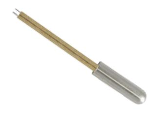
The RTD Probe—High Temperature is ideal for use in high temperature applications. The sensing element is encapsulated in a ceramic tube and stainless steel sheath, this protects the sensor from impact damage. The lead wire conductors are made of Nickel which provides corrosion resistance while the fiberglass over braid provides elevated temperature protection. These High Temperature probes are designed for quick process time response. Custom options are available for your application.
