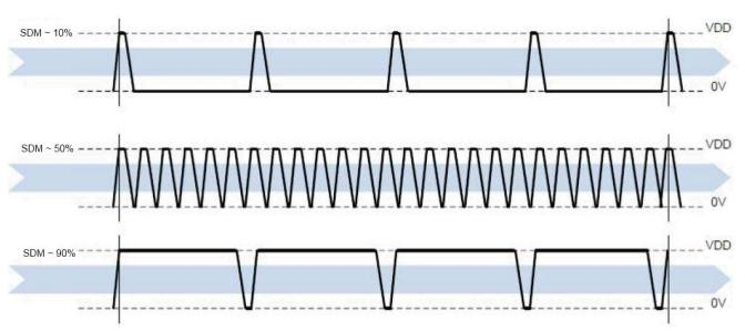
Sigma Delta Modulation output (SDM) is a bit-stream of pulses. The higher the pulse density is, the higher the measured temperature. The fundamental frequency of SDM is in the range of roughly 4 kHz and 65 kHz.
