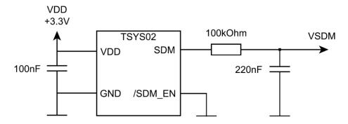
Recommended component values for a RC low pass are R = 100k $\Omega$  and C = 220nF. The resulting output voltage  $V_{SDM}$  represents the measured temperature with respect to  $V_{DD}$ .
