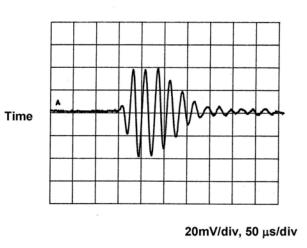
NOTE: Measured with PVDF transmitter (100Vp drive) and preamplifier (gain of 17)
