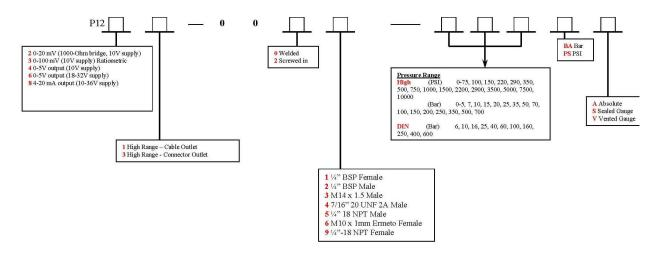
Example: P1283-0023-10KPSS = 4 to 20mA output, connector outlet, screwed in M14 male port, 10,000 psi sealed gauge
