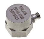
The Model 7514A is a stud mounted piezoelectric charge mode accelerometer with an operating temperature range to +260°C. The accelerometer is designed for high frequency vibration and shock measurements and offers a wide bandwidth to >14kHz with a nominal charge output of 50pC/g. The model 7514A features a hermetically sealed stainless steel housing and a #10-32 stud mount configuration.
