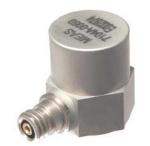
The Model 7504A is a stud mounted piezoelectric charge mode accelerometer with an operating temperature range to +260°C. The accelerometer is designed for high frequency vibration and shock measurements and offers a wide bandwidth to >10kHz and a nominal charge output of 5.6pC/g. The model 7504A features a hermetically sealed stainless steel housing and a #10-32 stud mount configuration.
