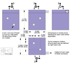
Two 3 mm x 0.5 mm threaded holes are provided on each of three orthogonal faces for mounting
