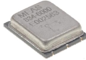
**The Model 834** is a low cost, board mountable triaxial accelerometer designed for high amplitude embedded shock applications. The accelerometer features a maximum current consumption of 4 micro-amps and incorporates full power and signal conditioning. The model 834 is available in  $\pm 2000g$  to  $\pm 6000g$  ranges and provides a flat frequency response up to 2kHz. The model 834M1 provides an extended frequency range to 6kHz.
