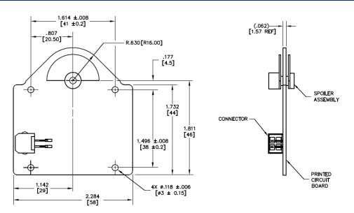
Dimensions are in inch [mm] Minimum area requirement 2 square inches, double sided PCB
