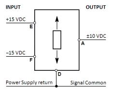
A through F: Connector pin assignments
